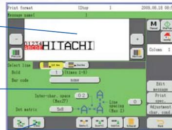
Various parameters, such as the line configuration and font size, can be easily set on a single screen.
